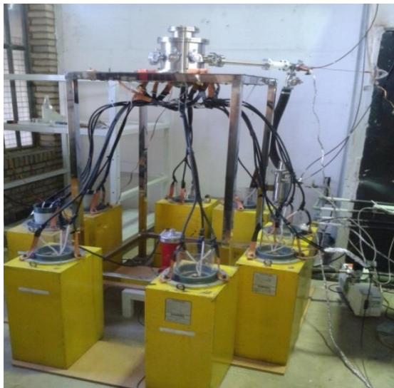
Fig. 2. Plasma focus 2.5Kj and its capacitors.
